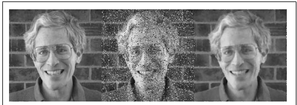
Figure 41: The original image on the left, the noisy image in the center, and the noisy image smoothed with a median filter on the right.
