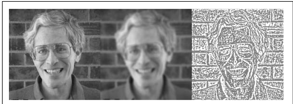
Figure 40: The original image on the left, the smoothed image in the middle, and the unsharp masked image on the right.
