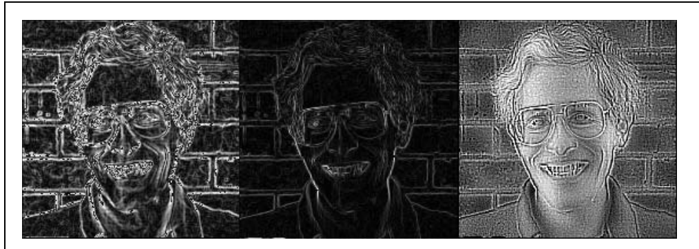
Figure 42: Three different ways to enhance the edges of images. On the left, the Sobel method. The Roberts method is shown in the center. Convolving the image with a Laplacian kernel is shown on the right.
